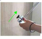
3. Insert the push plate into the clutch, return it to the shaft, and fix it according to the height of the bottle. (The felt side is on the bottom.)
