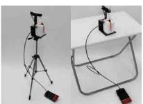
Use a stable table, desk, or tripod for the upper unit. Since there is screw hole for 1 / 4-20 UNIC screw on the bottom of upper unit, you can set to a tripod.
